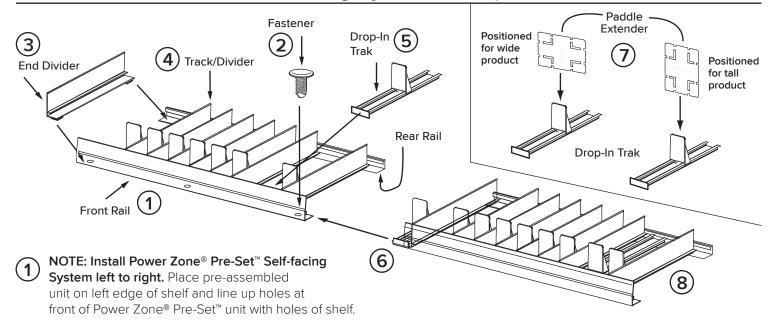
TIP: If front and rear rails are not even on the left-most part of the shelf, gently tap left end of Power Zone® Pre-Set™ unit on the floor to even them.
