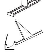
1 Insert front edge of Drop-In Trak under lip of front rail.
